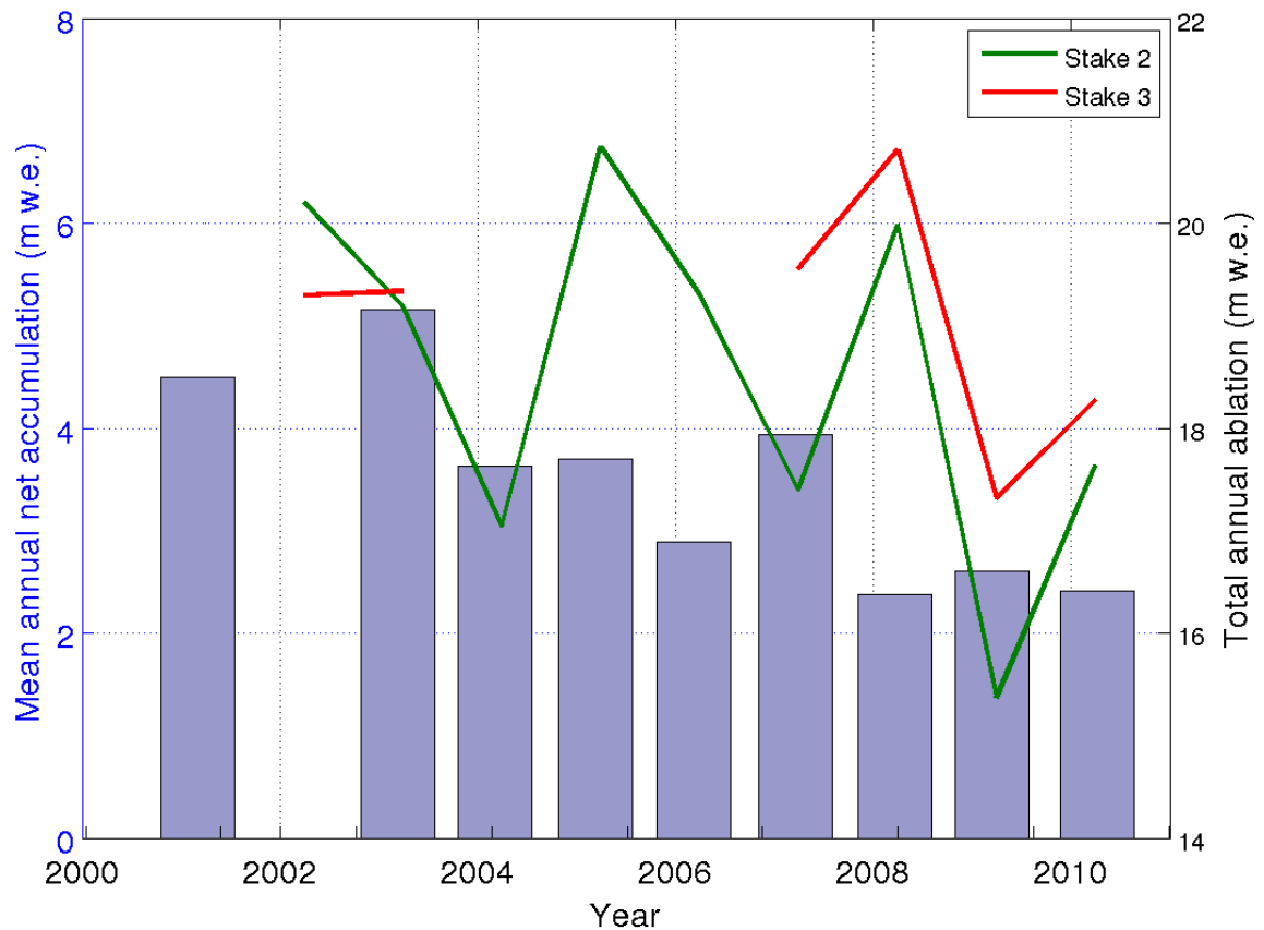
Figure 2. Inter-annual variation in mass balance measurements. Net accumulation measurements (blue bars) averaged over the accumulation area of the glacier show a generally decreasing trend after some high accumulation years at the start of the decade. Total melt at the terminus, measured using ablation stakes (red and green lines), show that the total melt is quite variable from year to year.
